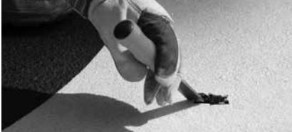
Chisel test to ensure proper bond.
