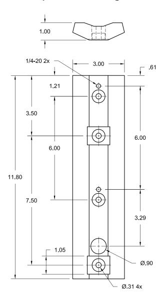
This adapter is designed to offset two Navigators on a 4" diameter pole so that two 9" x 12" signs can be mounted without conflict. One adapter is needed behind each Navigator. The adapters can either be strapped to the pole or bolted to the pole. For bolting, holes are provided to match 6" spacing of most push button signs or spacing for Pelco 5" x 7" frames if these types of frames were previously mounted.
