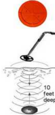
EMS locating markers (frequency needs to be defined) These can be molded into the cover of all pull boxes and vaults
