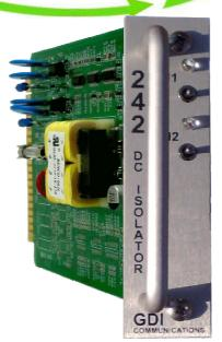
The GDI Model 242 Dual DC Isolator consists of two, independent, DC Isolators on one plug-in module. Each isolator converts a switch closure to a signal that a traffic controller can utilize.
