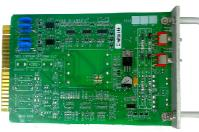
The **DIM242L** is configured to be powered from the +24vdc available on the 44-pin connector of the Input File.
