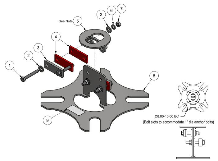
Note: First saddle #5 Conductor Guide onto #8 Cable Retainer Weldment before assembling #3 bar & #4 Pads
