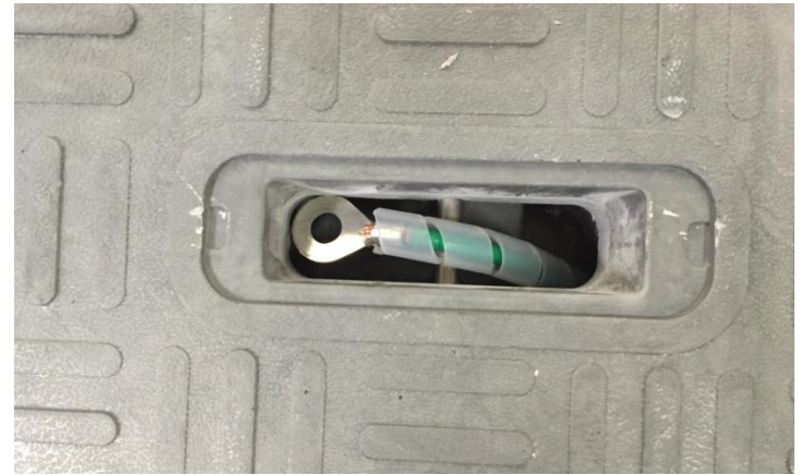
Figure 2 . Top View of Shield Lid with the un-covered Lift Pin Slot and 5' Ground Wire with Spiral Wrap in the stored position.
