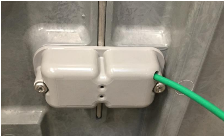
Figure 3 . Underside View of Lift Pin Cup with through hole for 5' Ground Wire.
