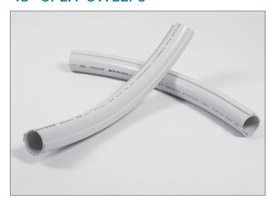
CRS's SPLIT SWEEPS are industry leading sweeps manufactured from CRS's SPLIT CONDUIT. They are great for 45 degree turns in the ground or for 45 degree risers coming up out of the ground. Just as with the SPLIT CONDUIT, when snapped together, the unique interlocking design of the SPLIT SWEEPS creates a smooth, tight seal protecting the cable or fiber optics from weathering.
