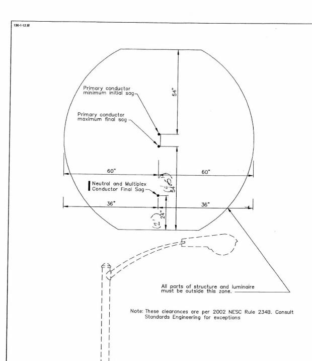
If the nearest powerline is closer than 10'away from the proposed pole location, KCPIL will need to sleeve the line during pole installation. They will invoice the City unless we call it out in the plans for the contractor to pay it.
