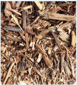
Filtrexx products are designed to Mimic Nature —we use an aged composted FilterMedia<sup>™</sup> (I) or Alternate FilterMedia<sup>™</sup> (r) inside a tubular mesh to harness nature's design principles of containment, filtration, retention, detention, energy dissipation, and vegetation establishment. As stormwater flows through the Soxx sediment and soluble pollutants are removed by:
