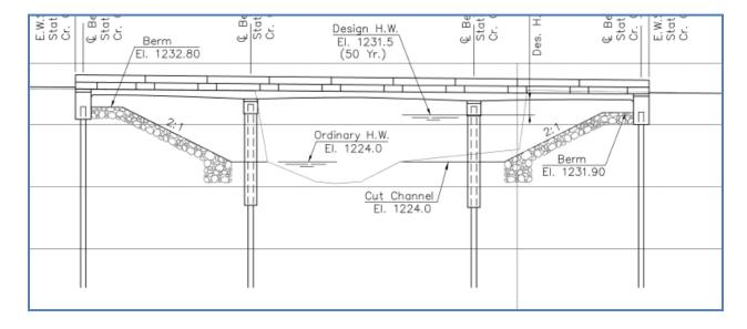
For grade separation bridges, the berm slopes will be protected as determined by analysis and any open ditches which convey drainage through the bridge will need to be maintained with the ditch bottoms receiving a minimum of a two-foot thick riprap lining.
