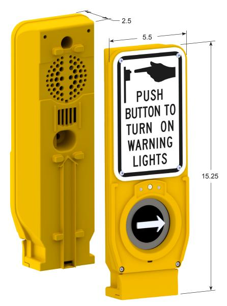
The XAV2E-LED push button station is designed for use at a pedestrian crosswalk with in-pavement or overhead flashing yellow lights. It works in conjunction with the XAVCU2 control unit. Within this system, the XAV2E-LED provides an instructional sign, a push button with directional arrow for activating the flashing lights, a voice message, and a group of three yellow LEDs above the push button which flash in sync with the street lighting.
