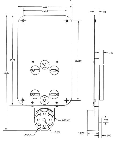
Polara Engineering's Push Button Frames are designed to mount on any pole from 21/2" up to 24" in diameter, or a flat surface. Their aluminum structure and powder coated finish provides a very strong and attractive mount for a pedestrian push button and sign.
