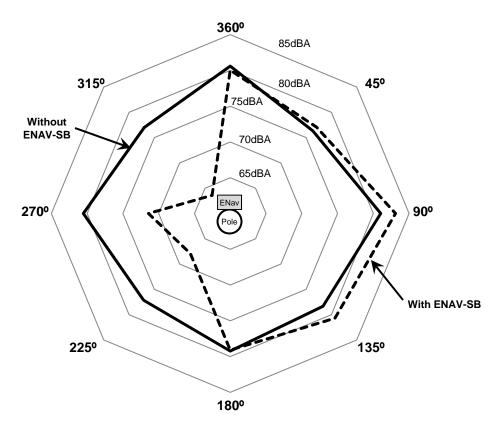
Comparison of audio levels with and without the ENAV-SB Sound Baffle
