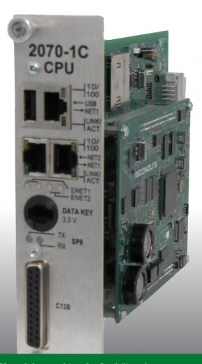
▷ ▷ The 2070-1C CPU and 2070-1CLS CPU modules combine the flexibility of open architecture hardware with the power and performance of our 2070 software packages.
