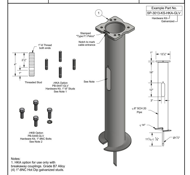
2. HKB option for use only with frangible breakaway base. ASTM A325 or Gr 5 SAE J469 (4) 1"-8NC x 3" Hot Dip galv Hex Hd
