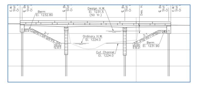
For grade separation bridges, the berm slopes will be protected as determined by analysis and any open ditches which convey drainage through the bridge will need to be maintained with the ditch bottoms receiving a minimum of a two-foot thick riprap lining.
